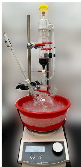
Figure 4. Assembled reaction set up for Step B
